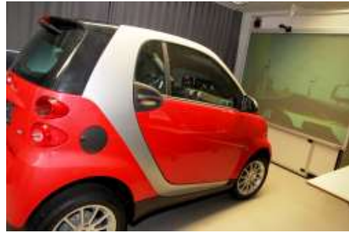
Fig. 3. (a) First prototype of DRIVE project in MR lab; (b) Second prototype of DRIVE project using real car as input device
