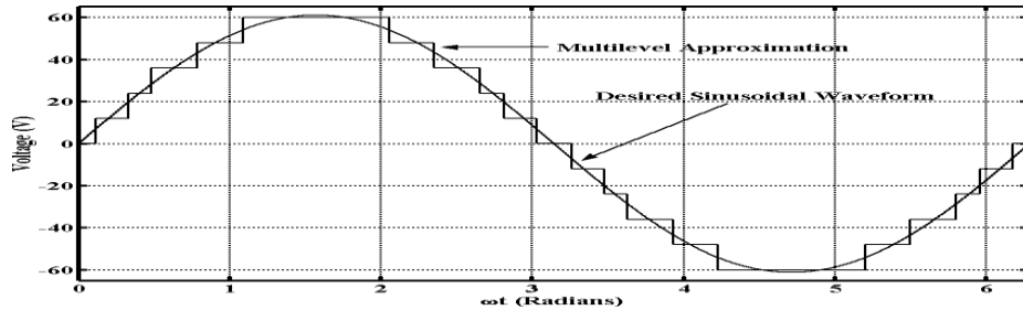
Fig.2 switching angle of multilevel inverter
