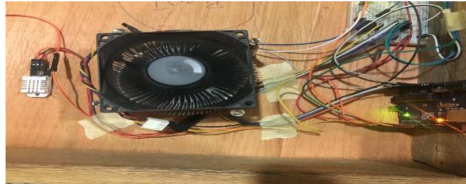
Fig 9: connection of DHT11 with Arduino
