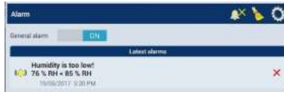
Figure 6. Notification shown when humidity is less than 85%RH.
