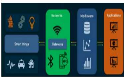
Figure 1. IoT communication architecture
