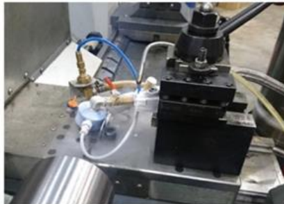
Fig 1: a) MQL supply with cryogenic
